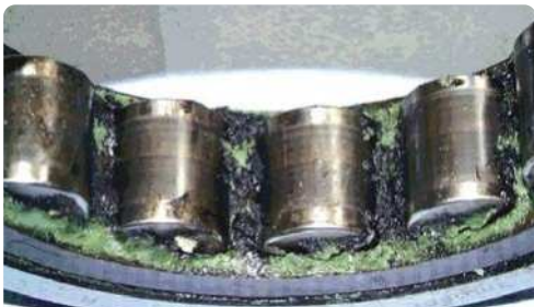
Lubricant degradation caused by electrical discharge currents
